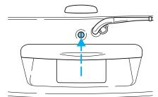
door locks, depress the key lock cylinder or press the door lock switch on the left side of the cargo area.
